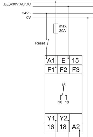
Range 300V with power modul 400V a.c. without fault latch
