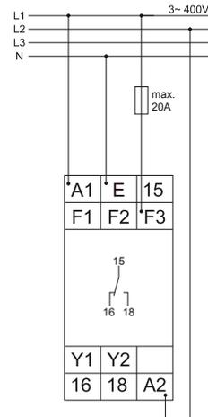
Range 60V with power modul 230V a.c. with fault latch
